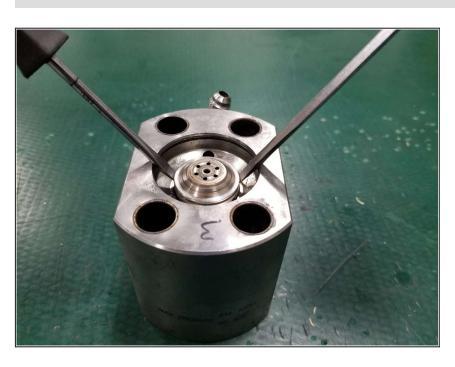
Carefully lift the check valve assembly using two flathead screwdrivers in the groove on the check valve body
